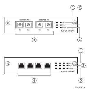
Figure 2. 100BASE-FX MDA Front Panels
